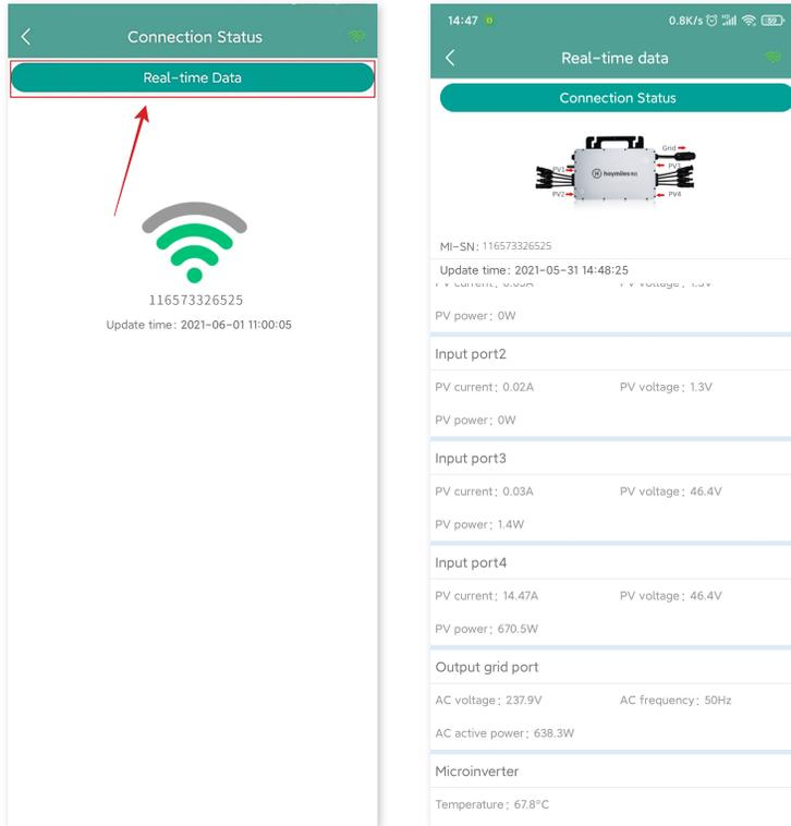
Note: If the microinverter has no signal, please check whether the microinverter is powered on or refer to the microinverter user manual for troubleshooting.
