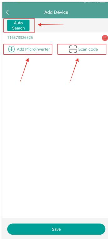
4. The search result of microinverters and microinverters added will be displayed in the list. Tap the button on the right if you want to delete it.
