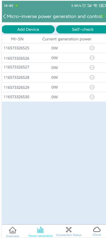
2. If you want to see more details of one microinverter, just click the serial number, then you can check the input and output data on the page shown as below.
