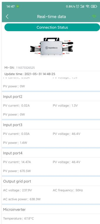
**Note:** If the microinverter signal is so weak that the real-time data are not updated, move the DTU closer to the microinverter.
